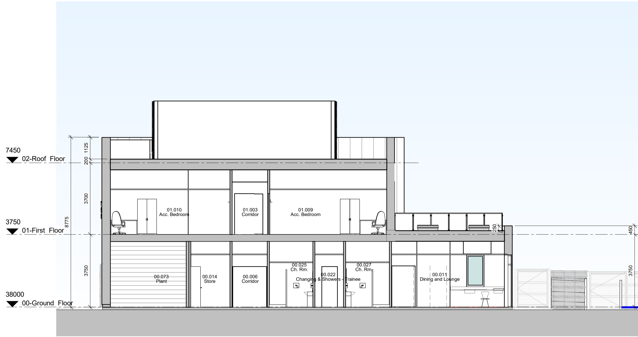
A Building Section A 1 : 100
