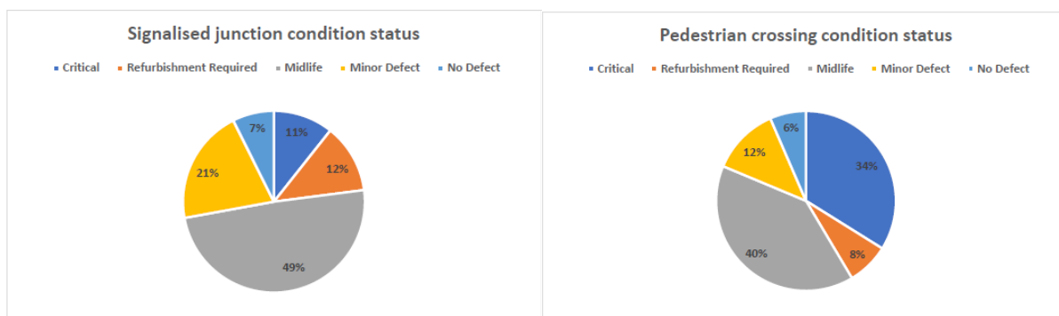
Overall Traffic Signal, Pedestrian Crossing Asset Condition (April 2020) Fig. 7 & 8
